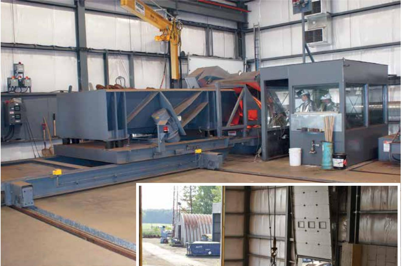
Fonderie Laperle invested in a new building addition to house its charging area (right), melt deck (above) and transfer car.
