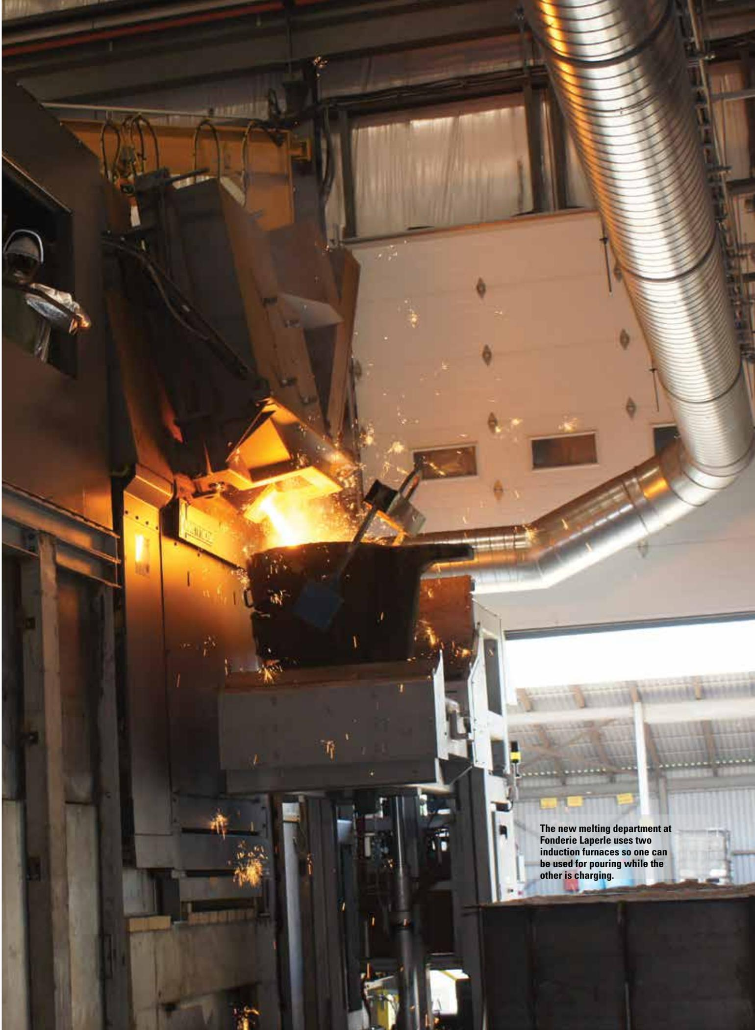
The new melting department at Fonderie Laperle uses two induction furnaces so one can be used for pouring while the other is charging.
