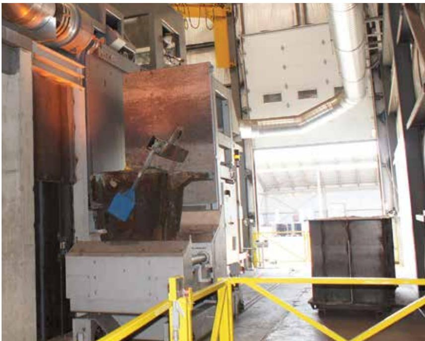
An automated transfer car carries a recently filled crucible from the furnace to the molding line for pouring.
